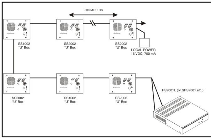
**FIGURE 5.** A 2-channel Audiocom intercom system using a PS2001L power supply.
